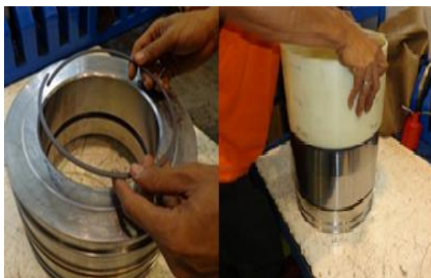
Figure 22. Installing Cushion Bearing
