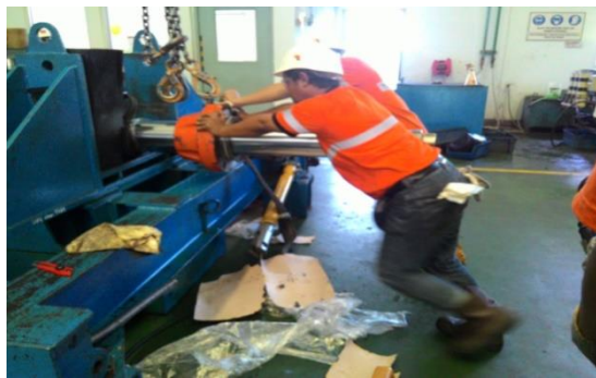
Figure 12. Disassembling the Head Cylinder
