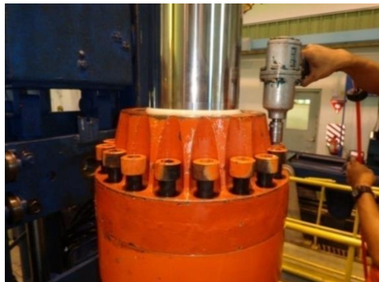
Figure 27. Tightening the Cylinder Head Bolts
