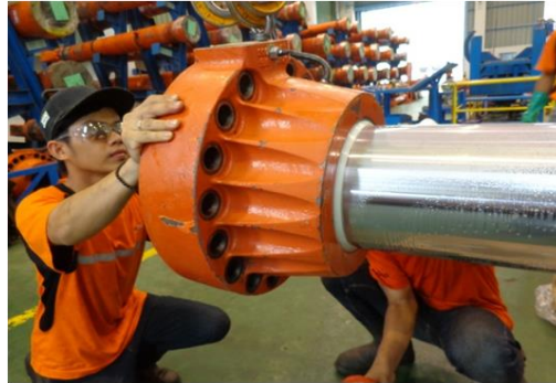
Figure 18. Assembling Cylinder Seal Head
