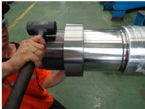
Figure 21. Installing Cylinder Head
