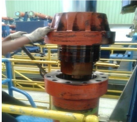
Figure 8. Disassembling the Cylindrical Boom Source: Personal Documentation of Researchers
