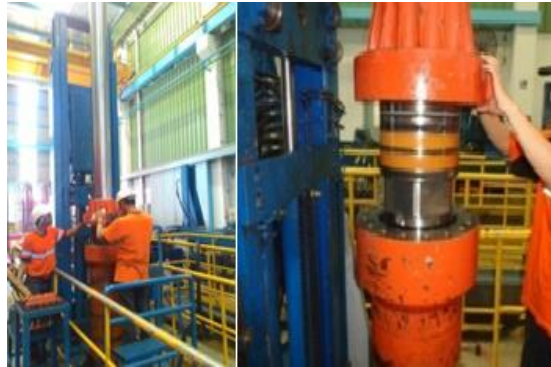
Figure 26. Assembling Boom Cylinder
