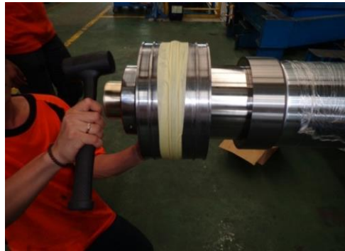
Figure 24. Tightening the Nut
