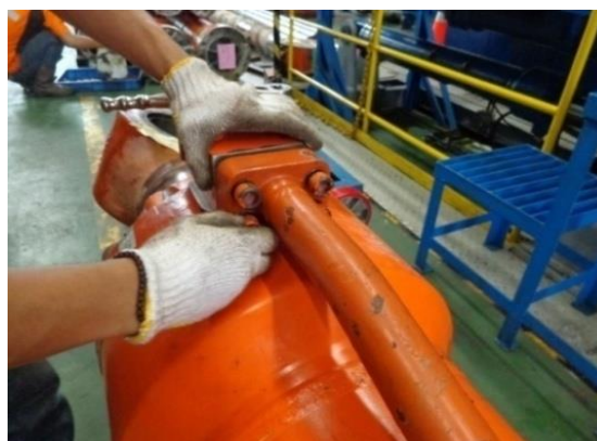
Figure 28. Assembling the Slow Return Valve
