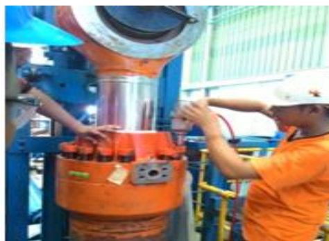
Figure 7. Removing The Cylinder Head Bolts
